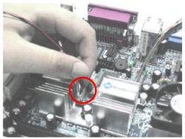
5. Connect the panel power cable, one side onto the LVDS-01 (+12V\_CONN) and the other side onto the FAN3 connecter on the motherboard.
