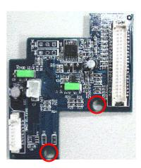
2. Line up the screw-fixing holes of the RGB-01 module with the screw-fixing holes on the Dual heatsink. The screw-fixing holes are indicated by red circles above.
