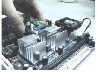
3. Fix the screws to the indicated holes. For each hole, add a washer in between the module and the heatsink.
