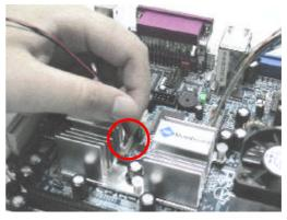
5. Connect the panel power cable, one side onto the RGB-01 (+12V\_CONN) and the other side onto the FAN3 connecter on the motherboard
