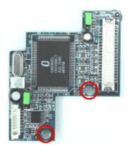
2. Line up the screw-fixing holes of the LVDS-01 module with the screw-fixing holes on the Dual heatsink. The screw-fixing holes are indicated by red circles above.
