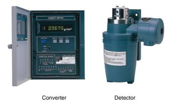
Measuring liquid temperature: -10 to 100 °C Measuring liquid pressure: 2 MPa G or less Withstandable pressure: 4.9 MPa G Steam tracing: Available Process connection: Rc1/4 Electrical connection: G3/4 Mounting: JIS 50A pipe mounting Ambient temperature: -10 to 50 °C Weight: Approx. 12 kg
