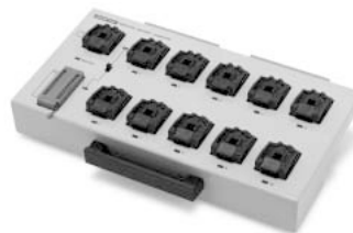
R49515B 1M- to 8M-bits For 32-pin PLCCs For master devices (32-pin lever socket × 1 and 32-pin PLCC socket × 1)
