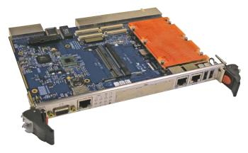
Diversified Technology's CPB4811 PICMG® 2.16-compliant packet switched backplane (PSB) processor blade combines high performance with low power for telecom and Internet IP-based applications.
