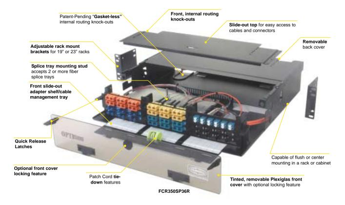
The OPTIchannel FCR Rack Mount Fiber Patch Panels provide superior fiber cable management and patch cord protection while allowing quick and easy access to connectors and splices. Available in 2, 3, or 4 rack unit heights, these panels have been designed with innovative features for both the cable
