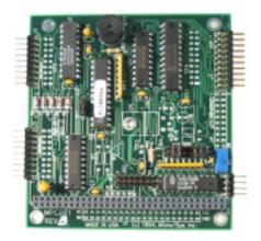
The MPC201 LCD and keypad interface allows direct connection to alphanumeric LCD displays (i.e. 2 line by 40 character, etc.). In addition, sub-VGA graphic LCD displays can also be driven if they employ an 8-bit parallel interface.
