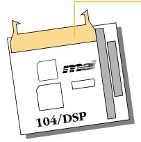
NOTE: One axis connection shown; 100-pin high-density connector supports up to 4 axes
