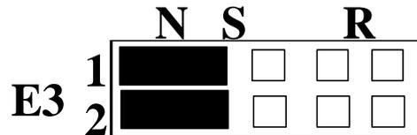
Figure 3 - Header E3, Normal IRQ Mode
