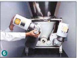
Reposition motor and drive assembly. Tighten swivel assembly bolt, replace back panel cover, and you're ready to run – all in under two minutes.
