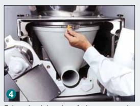
Release band clamp lever for hopper removal.
