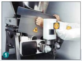
All internal components are accessible from the rear of the feeder instead of the discharge side. Simply remove back panel and loosen swivel assembly bolt.
