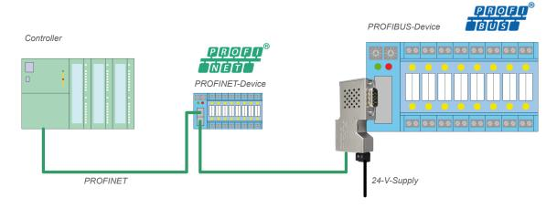
netLINK PROXY is plugged directly onto the PROFIBUS-DP connector of the slave. It is powered by 24 V. The RJ45 PROFINET jack is to be connected to PROFINET. The PROXY is configured via a PC with the configuration tool suite SYCON.net. The DP-slave configuration data is identified by scan and GSD file. Based on this configuration SYCON.net generates a GSDML file for the PROFINET controller configuration.
