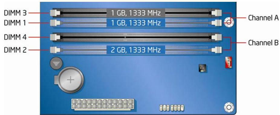
Figure 14. Example Dual Channel Memory Configuration with Three DIMMs
