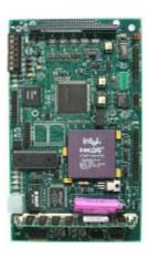
Netsock/400 provides a turnkey, network-oriented platform on which to build embedded systems. Based on the Micro/sys SBC2486DX embedded PC and its built-in 10BASE-T Ethernet port, Netsock/400 is a powerful 486DX computer that offers high performance, and that can significantly reduce development time.
