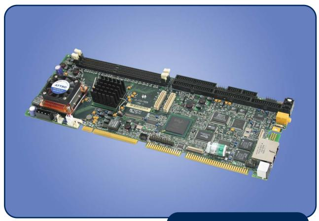
The feature-rich MAT 1100 PICMG® single board computer combines powerful Pentium® M processor technology with the Intel 855GME chipset. Video support, provided by the on-board integrated 855GME graphics controller, can be further enhanced via the optional VID998 and VID1080 AGP daughter cards. Both offer high performance video options and support the nVidia® Geforce2 and ATI 7500 and 9000 controllers respectively. Features include dual display architecture, DFP/LVDS support and video capture.
