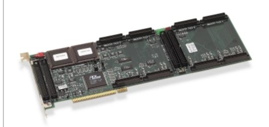
PCI-40A is an IndustryPack® carrier board that provides four IndustryPack slots on a single desktop or industrial PCI slot card. The IndustryPack bus clock is software-selectable on a per-slot basis between 8 and 32 MHz.
