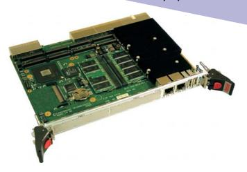
monitoring is provided by the PICMG 2.9 compliant IPMI interface. To simplify the board's integration many popular industry standard operating systems are supported. The PP 332/02x-U is suitable for a range of applications within the industrial control, telecomms, telemetry, scientific and aerospace markets. The PP 332/02x-U is the RoHS compliant version of the PP 332/02x family.
