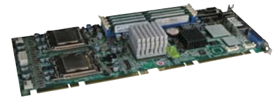
PICMG 1.3 Processor Board based on the Intel® Xeon Dual-Core or Quad-Core LGA-771 package
