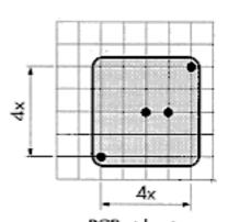
PCB side view: Pitch: x = 2,54 mm 0,8 mm diameter hale
