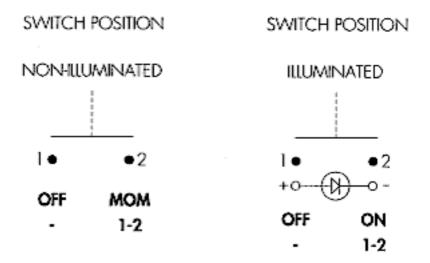
1-pole, 2-position COSMOS key switch Independent LED circuit
