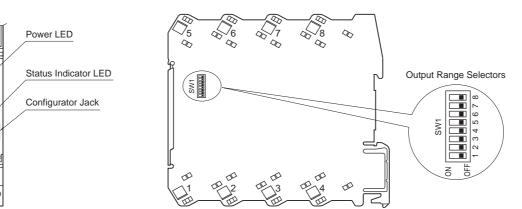
The output signal type is configurable with the DIP switches. Refer to the installation manual for detailed procedure.
