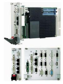
The F8 is a powerful CompactPCI or busless industrial PC for multimedia and infotainment applications -- for vehicles (railways, buses, planes, trucks...) and stationary information systems. It is designed to operate in harsh environments up to EN 50155 (railway standard).
