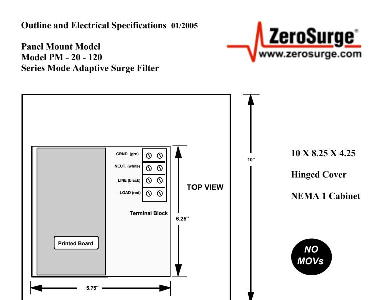
This model has been optimized for protecting switch-mode power supplies (used in computers and most newer electronic equipment).
