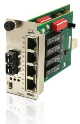
The ION 4xT1/E1/J1 copper to fiber network interface device (NID) provides a solution for those users that need to extend multiple T1/E1 connections over fiber.
