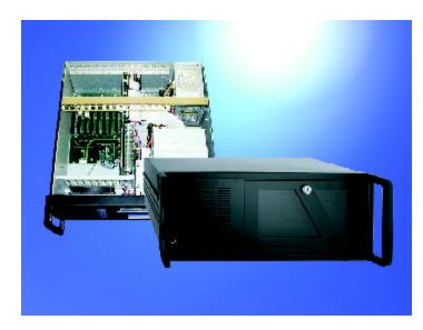
The Nd61400 industrial computer features choice of a 1.2 GHz Pentium III or 2.4 GHz P4 CPU plugged into a 14-slot backplane with eight (8) ISA, four (4) PCI and two (2) PICMG slots (other slot combinations are available). This industrial PC is intended for processorintensive applications requiring high-reliability in an industrial environment. The Nd61400 is available in 4U rack mount configuration with front-accessible floppy, CD-ROM and removable hard drive.
