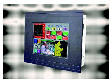
Intended for all applications requiring high reliability in a small package, the DisplayPac-OP industrial computer features a choice of computing engine up to 2.8 GHz, choice of display size 12.1", 15" or 17" active matrix TFT LCD, resistive touchscreen, hard drive, floppy, CD-ROM, two PCI expansion slots (one shared ISA) and an internal power supply in a heavy-duty steel enclosure. It is FCC, CE and UL approved and rated to operate from 0° - 50°C at 10 - 90% humidity.
