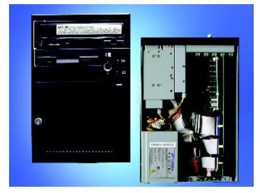
The Nd60501 industrial computer features either a 1.2 GHz Pentium III or 2.4 GHz P4 CPU plugged into a 6-slot backplane with four (4) PCI, one (1) ISA and one (1) PICMG slot. This industrial PC is intended for processor-intensive applications requiring high reliability in an industrial environment. The Nd60501 is available in desktop or wallmount configuration with front-accessible floppy and CD-ROM.
