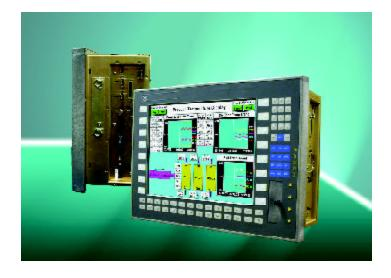
The Panel C features a bright 15" XGA active matrix color TFT LCD, and is powered by a Pentium III 1 GHz processor with up to 512M RAM. Built-in numeric keypad, side keys (PC control and CNC), and function keys (Fx and Alpha) provide human-machine interface. Status LEDs indicate power, run, fault, etc. The unit features a 40gigabyte hard disk drive for data storage.
