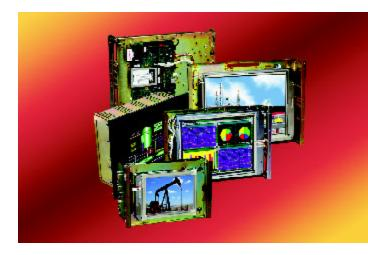
The DisplauPac-ARM is a family of products designed specifically for embedded operating systems. Powered by an Intel StrongARM SA-1110 206 MHz sinale board computer, the sustems offer low-power operation while providing high-powered processing. In addition to 64M Synchronous DRAM and 32M Flash memory, the systems provide a type II PCMCIA socket for additional storage capacity or I/ O modules such as GPS or wireless Ethernet. A CompactFlash socket provides yet a third option for storage media.
