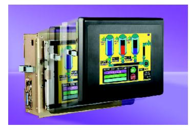
The DisplayPac-Access features a 10.4" or 12.1" SVGA active matrix TFT LCD, a Celeron or Pentium III computing engine with PC/104 expansion, a resistive touchscreen and optional keypad. The sturdy enclosure design features quick-release latches which let the user easily detach the computer and display portion from the touchscreen and front bezel. This simple access permits quick onsite maintenance, system upgrades, software changes and field replaceability of backlights.
