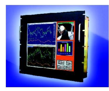
The ThinView-18-RM flat panel monitor with an integrated resistive touchscreen features an 18.1" active matrix color TFT LCD. It has a NEMA 4 rating on the front surface, with the front bezel ready to be rack mounted to your 19" rack-mount equipment. The rack-mount bezel is constructed of powder coated metal with a fingerprintproof, clear plastic overlay. The anodized aluminum rear cover is vented for heat dissipation and provides protection for all electronics.
