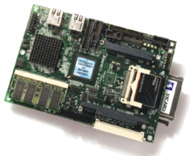
The PCS-620 operates from  $-40^{\circ}$  to  $70^{\circ}$  C, or from  $-40^{\circ}$  to  $85^{\circ}$  C at lowered clock speed.
