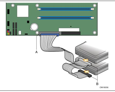
Figure 16. Connecting the IDE Cable
