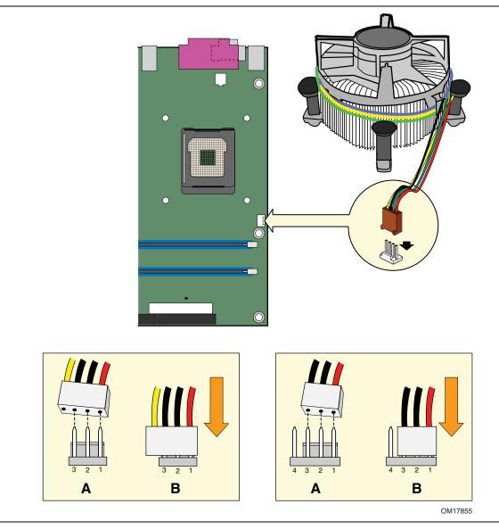
Figure 12. Connecting the Processor Fan Heat Sink Cable to the Processor Fan Connector
