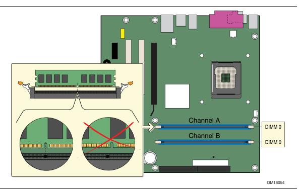
Figure 14. Installing a DIMM
