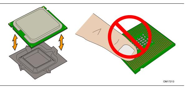
Figure 9. Remove the Processor from the Protective Processor Cover/Do Not Touch
