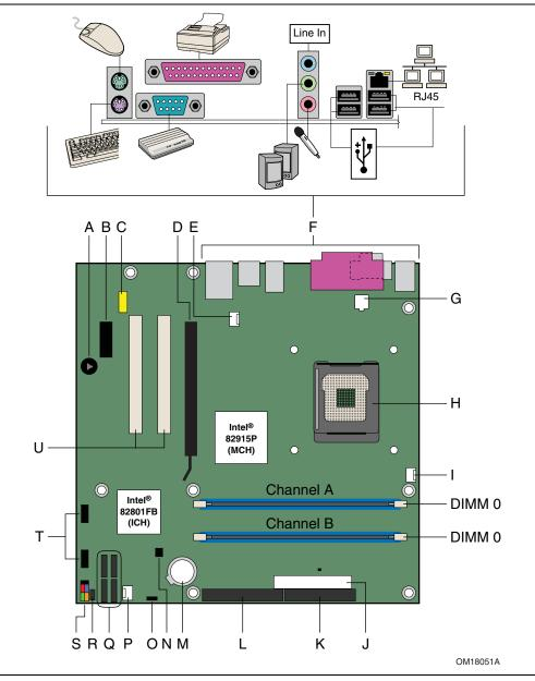
Figure 1. Intel Desktop Board D915PDT Components
