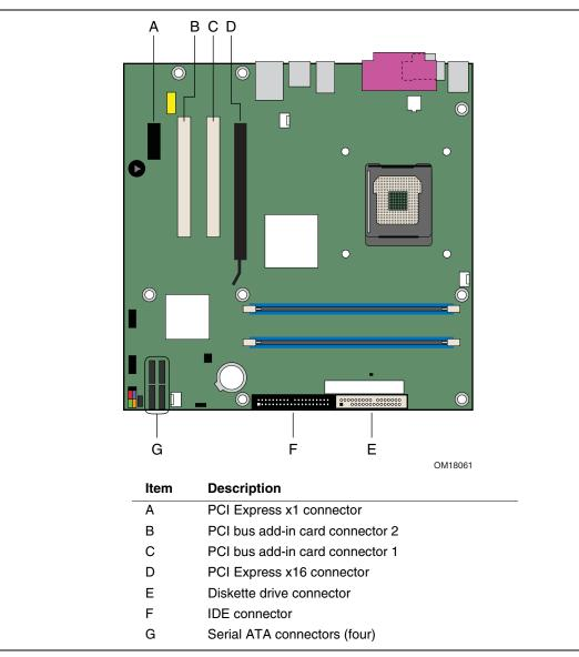
Figure 22. Location of the Other Connectors on Desktop Board D915PDT
