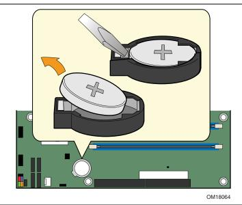
Figure 25. Removing the Battery
