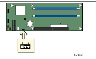
Figure 23. Location of the BIOS Configuration Jumper Block
