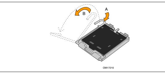
Figure 6. Lift Socket Lever
