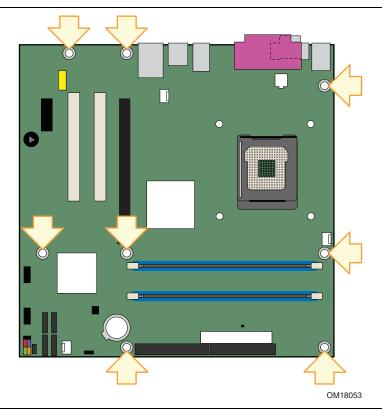
Figure 5. Desktop Board D915PDT Mounting Screw Hole Locations
