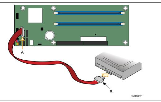
Figure 17. Connecting the Serial ATA Cable
