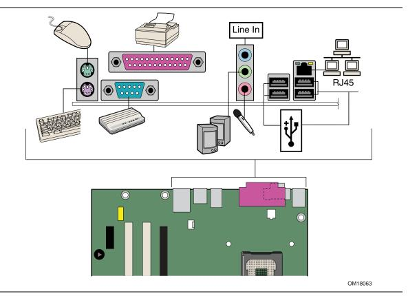
Figure 24. Back Panel Connectors
