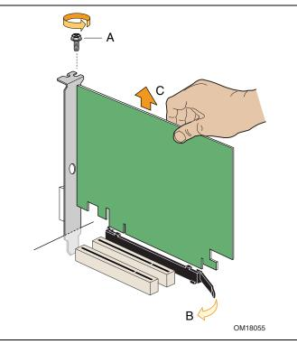
Figure 15. Removing the PCI Express x16 Card
