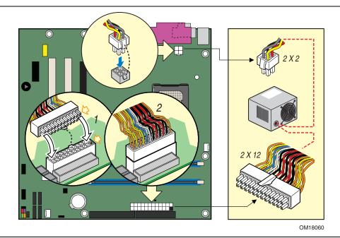
Figure 21. Connecting Power Supply Cables
