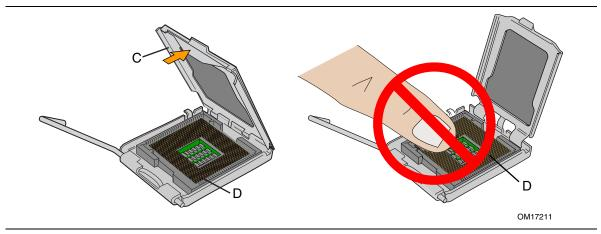
Figure 7. Lift the Load Plate and Don't Touch the Socket Contacts
