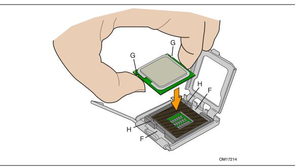
Figure 10. Install Processor
