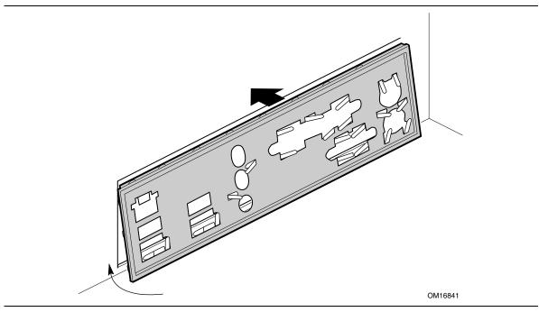
Figure 4. Installing the I/O Shield
