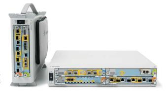
Wire-speed traffic generation, routing protocol emulation and analysis for the development and deployment of routers and switches with 10 Gb/s Ethernet or Packet over SONET/SDH interfaces.
