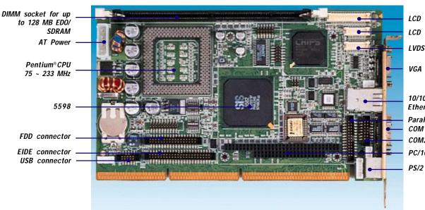
LCD connector 36-bit LCD connector 18-bit LVDS out 18-bit
