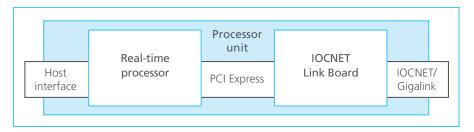
The real-time PC of the Processing Unit is extended by an IOCNET Link Board to connect it to the SCALEXIO system.
