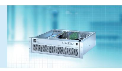
The SCALEXIO processor core is based on an industry PC with an Intel Core i7 quad-core processor, a real-time operating system (RTOS), and a PCIe plug-on card developed by dSPACE for communication with the I/O and with other real-time processors. Because standard components are used
