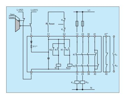
Example for dual-channel door monitoring using two limit switches (one with positive opening contacts) and external reset button.
