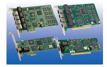
The Diva BRI offer voice, speech, conferencing, VoIP, modem and fax features, and can serve as a base for many communication applications. The boards support most standard applications, and are also suitable for new application development. The Diva BRI are available in Low Profile or Half Size form factors. The Diva BRI can be seamlessly combined with other Dialogic<sup>®</sup> Diva<sup>®</sup> Media Boards, such as analog, E1/T1, ISDN PRI, and VoIP.
