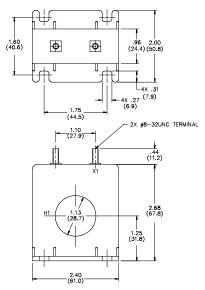
Part Number: CT005001 Current Ratio: 50: 0.1 (Amperes) Operation Frequency: 50 to 400 Hz
