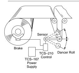
The complete system consists of five components:
