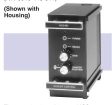
The completely solid state MCS-203 Dancer Control Module is designed for automatic web tensioning through the use of a dancer roll. The MCS-203 can control two 24 VDC tension brakes in parallel. It works on the concept of a P-I-D controller and has internal P, I & D adjustments for optimum performance regardless of brake size.
