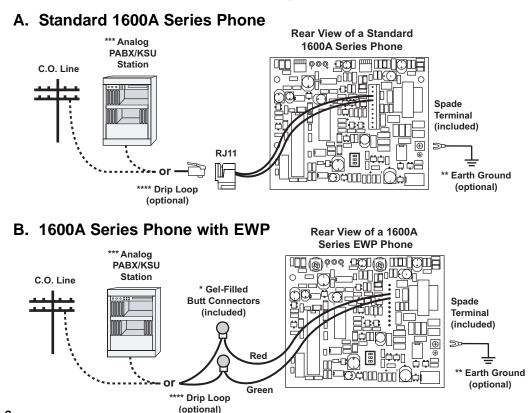
IMPORTANT: Electronic devices are susceptible to lightning and power station electrical surges from both the AC outlet and the telephone line. It is recommended that a surge protector be installed to protect against such surges. Contact Panamax at (800) 472-5555 or Electronic Specialists Inc. at (800) 225-4876.
