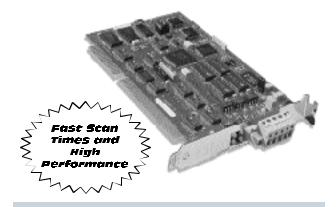
The SST DeviceNet Pro ISA card connects your ISA bus computer to DeviceNet. The Pro Card is a high-performance version of the SST DeviceNet ISA card and is compatible with all applications written for the SST DeviceNet ISA card.
