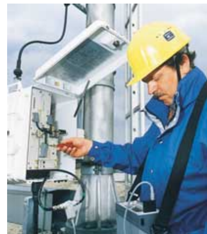
Level Meter URV35 with Insertion Unit URV5-Z2 in mobile use
