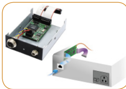
Stand-alone Type (Pin header Ethernet, NE-4110 Series)
