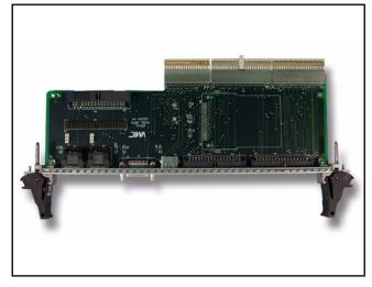
**Power Requirements:** Power for the VMIACC-0576 is +5 V, supplied through the J3 connector on the CPCI backplane.
