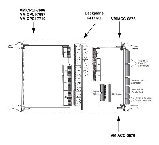
Figure 1. VMIACC-0576 and Rear I/O with VMICPCI-7696, -7697, or -7710
