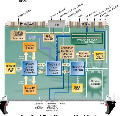
PowerNode5 Block Diagram and Front Panel
