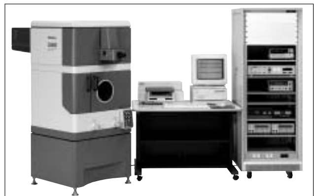
Interferometer as the standard for Gauge Block calibration (At Miyazaki Plant)
