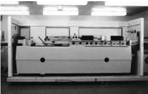
Interferometer as the standard for Linear Scale calibration (At Kiyohara Plant)
