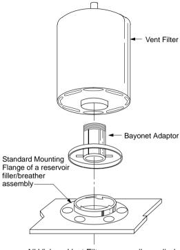
All Vickers Vent Filters are easily applied to reservoirs via Spin-On adaptors.
