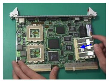
2. When the gold finger of the memory module is completely slid into the socket, push the memory module onto the clip of the socket. With two clicks, the memory module is firmly held by SO-DIMM socket.
