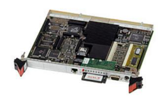
The D2 is a Pentium single-board computer optimized for industrial requirements in control and instrumentation in terms of functionality, environmental conditions and cost. It needs only one slot in a CompactPCI system. Its "Socket 7+"-based computing core supports Tillamook CPUs up to 266MHz. The chip set comes with 100MHz CPU and 33MHz PCI bus clock and supports the latest DRAM technology. All PCI components are carefully selected for optimum support regarding long-term availability.
