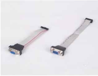
P/N 1701160150 VGA cable D-SUB 15-pin to IDC 2 x 8-pin pitch : 2.0 mm, L = 15 cm
