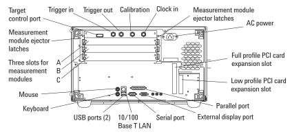
Figure 18. Agilent 16903A back panel
