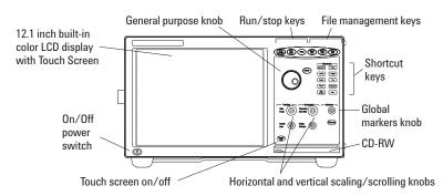
Figure 15. Agilent 16902A front panel
