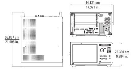
Figure 12. 16900A/16902A/16903A exterior dimensions
