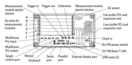
Figure 14. Agilent 16900A back panel
