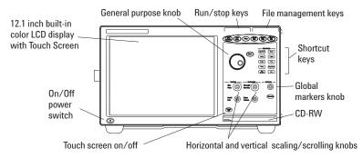
Figure 17. Agilent 16903A front panel
