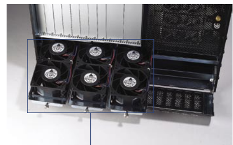
Six 80-CFM front-access hot-swappable fan modules
