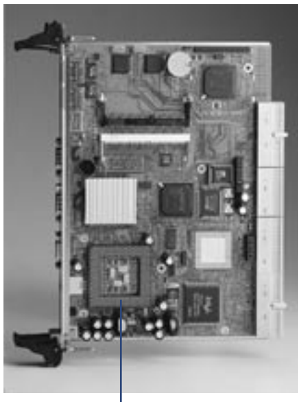
Socket 370 Pentium III/Celeron CPU
