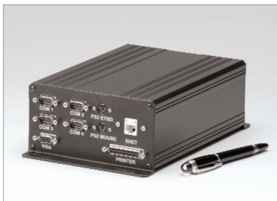
Enclosure for EPIC single board computers
