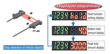
Press and hold setting switch for 5 seconds
