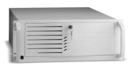
14-slot passive backplane up to 12 PCI slots or 64-bit 12 PCI passive backplane
