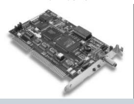
The SST Modicon ISA card connects your ISA bus computer to Modicon's Quantum and 800 Series Remote I/O on the S908 network.
