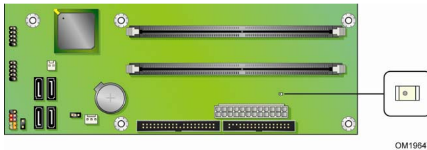
Figure 3. Location of Standby Power Indicator
